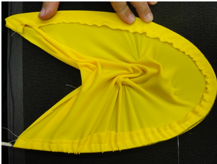
Figure 5: Reaction of elastane in the face of imposed stresses by tension and the stitch pattern.
