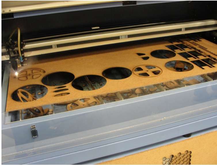
Figure 11. Cutting of the pieces to the movement mechanism of the physical model in laser cutter machine.
