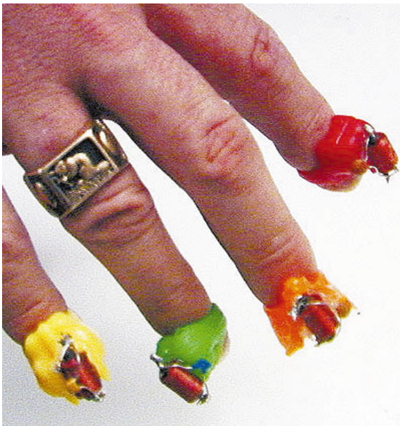
Figure 18 Small LC tags built into rings for efficient, wireless finger control
