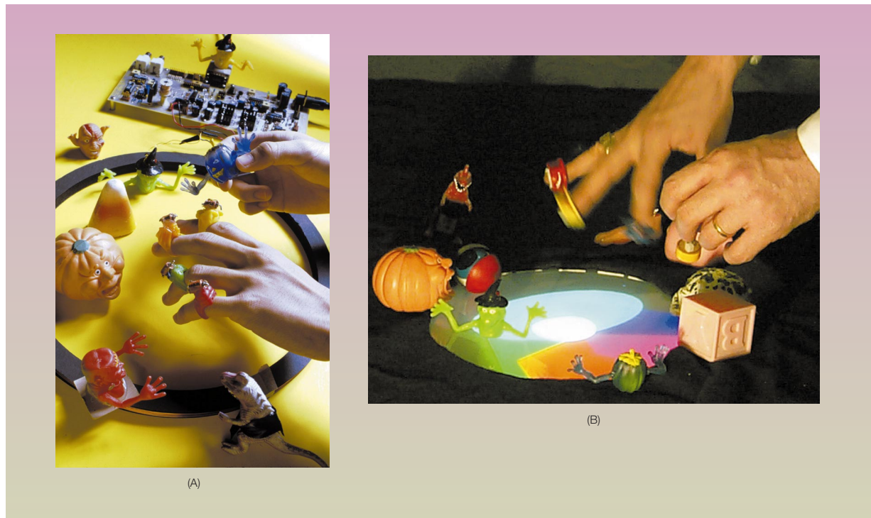
Figure 20 Musical Trinkets demonstrations (A) with many tagged objects, prototype reader hardware and reader coil and (B) in action with interactive graphics
