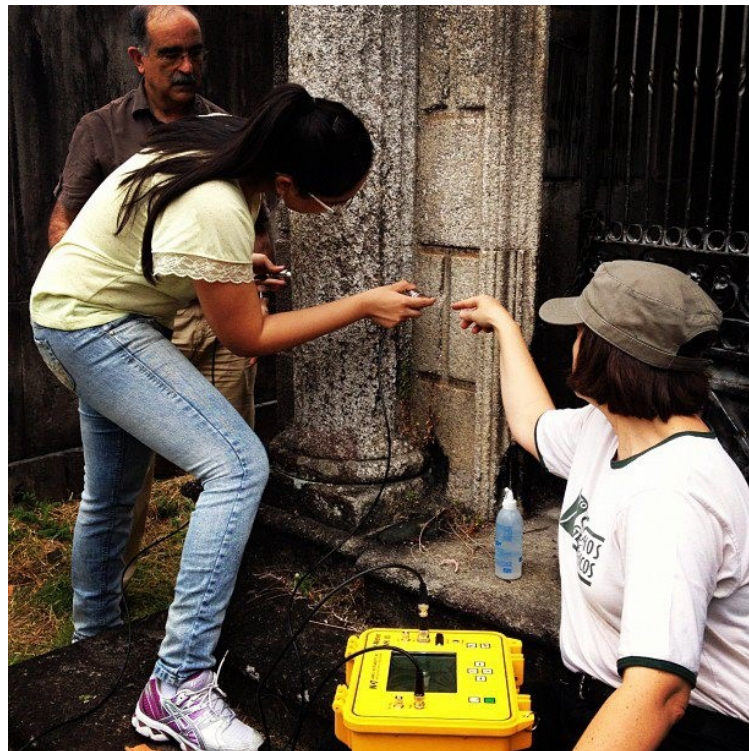
Fig. 3: Ultrasound analysis of the tomb granite column in Soledade during Pâmela Anne Bahia master dissertation field research, guided by Prof. Thais Sanjad, with research Del Lama (University of São Paulo) and José Delgado Rodrigues (National Laboratory of Civil Engineering / Lisbon), which guided these data collection. Cemetery Nossa Sen Soledade, Belém. Source: Thais Sanjad, 2013.
