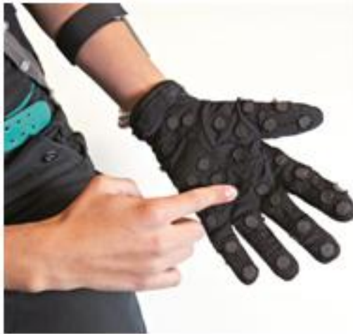
Figure 1. Input unit on the palm of the glove.
